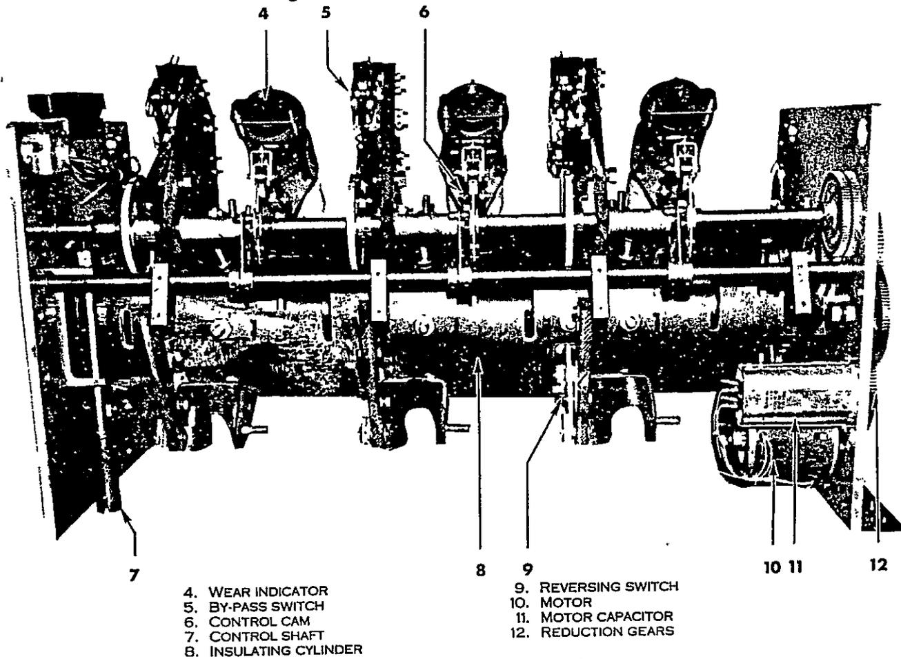
**Fig. 3. Rear view of switch mechanism**
