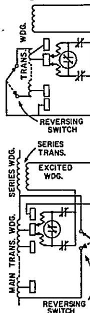
transformer should never be opened, as dangerously high voltages may develop! These voltages can not only break down insulation and destroy the current transformer but present a serious hazard to personnel.
