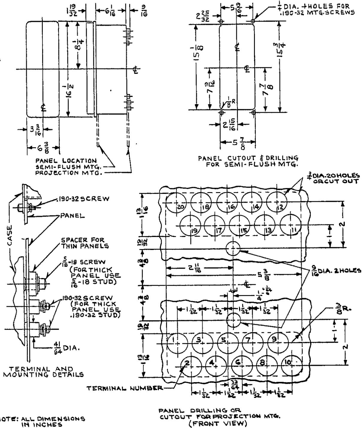
Fig. 13. Outline & Drilling Plan for the Type CA-6 Relay in the type FT-32 Case.
