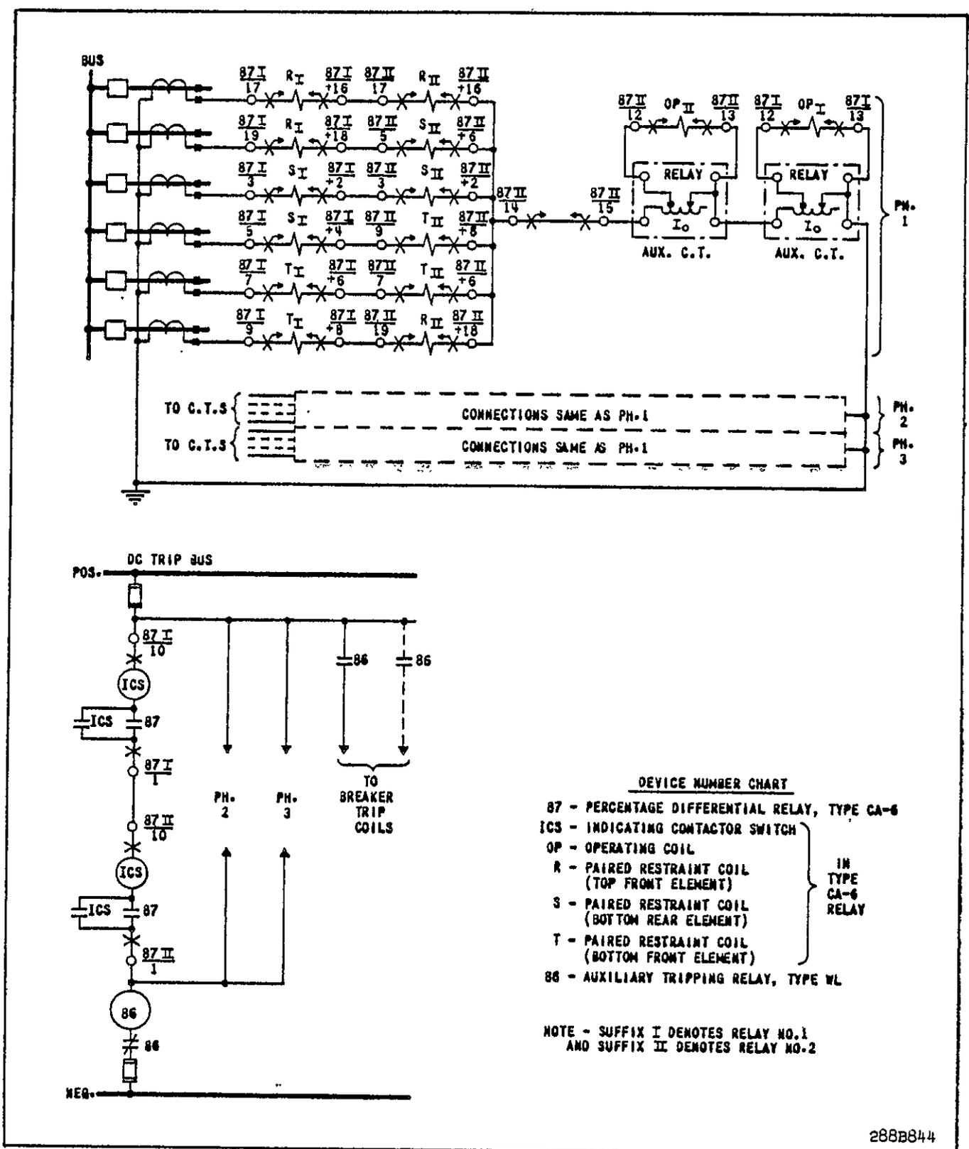
Fig. 8. External Schematic of Two Sets of Type CA-6 Relays for Six Circuit Bus Protection.
