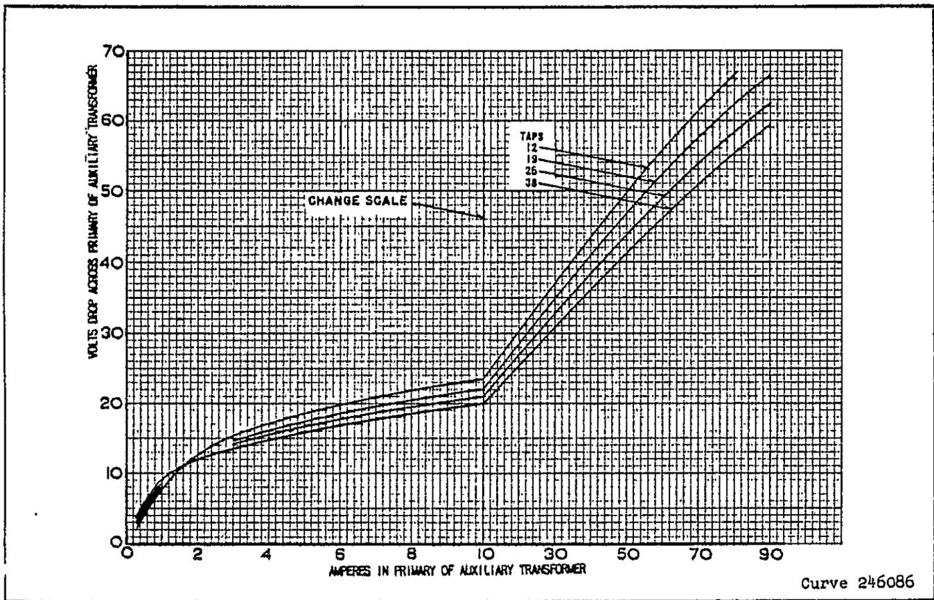
Fig. 5. Typical Burden Characteristics of The Operating Coil Circuit
