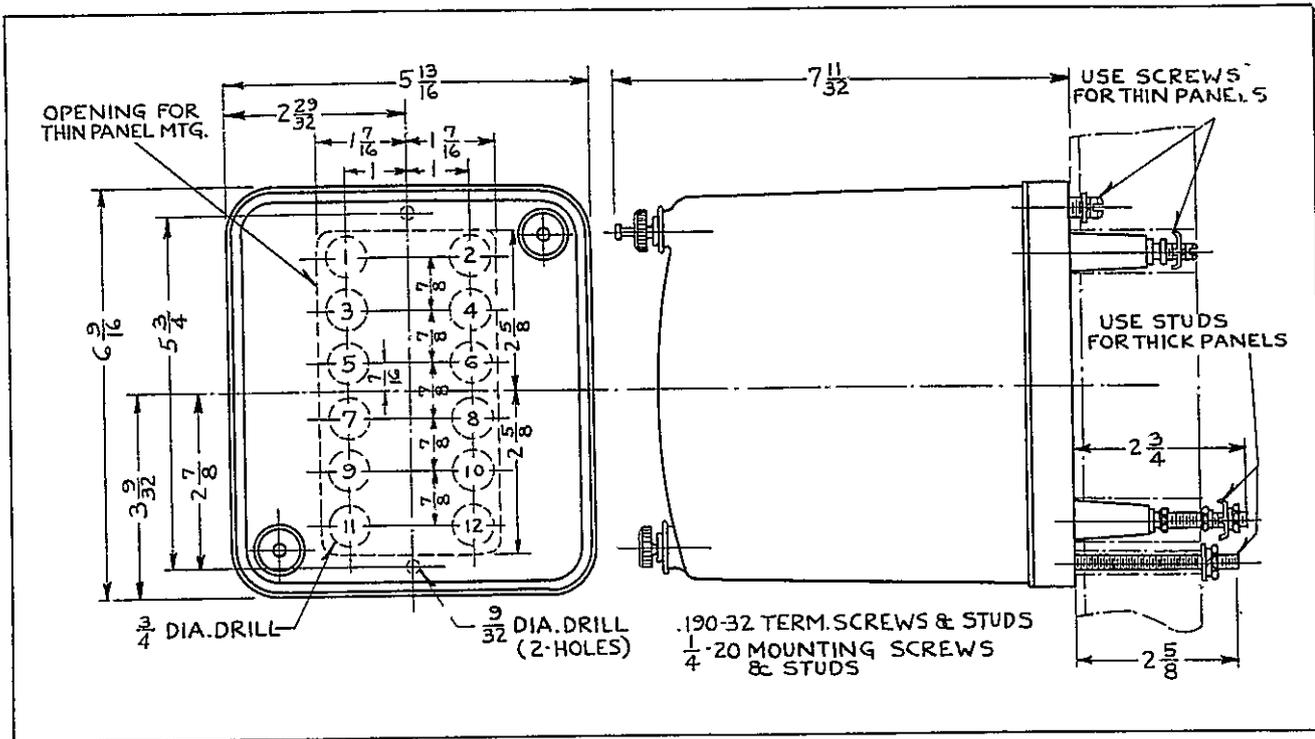
Fig. 12—Outline And Drilling Plan For The Standard Projection Type Case. See The Internal Schematics For The Terminals Supplied. For Reference Only.
