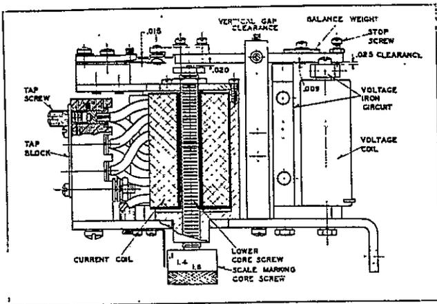
Fig. 1—Sectional View Of The Impedance Element.
