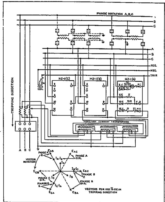
Fig. 11—External Connections of the Type HZ-1 Relay In The Type FT Case Using The Auxiliary Star-Delta Current Transformer.
