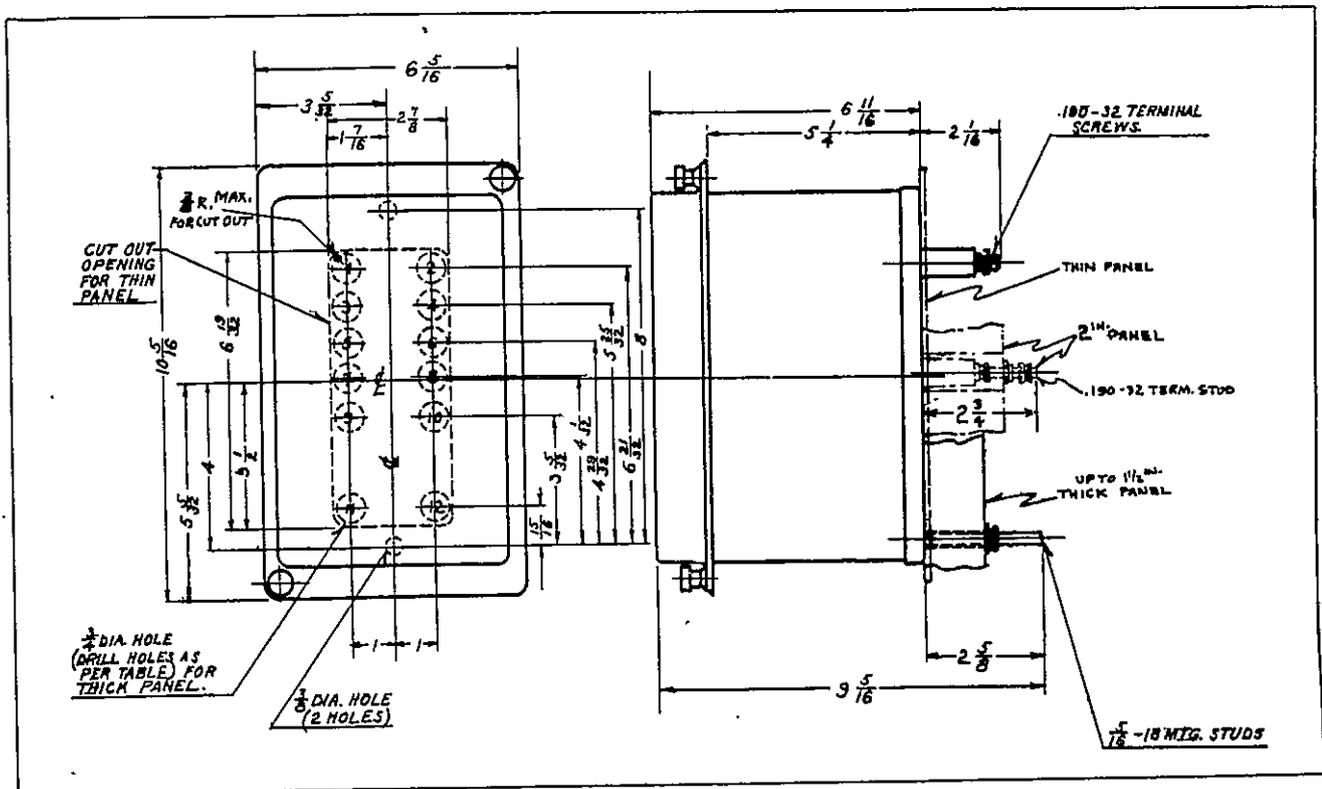
Fig. 13—Outline And Drilling Plan For The S10 Projection Type Flexitest Case. See The Internal Schematics For The Terminals Supplied. For Reference Only.
