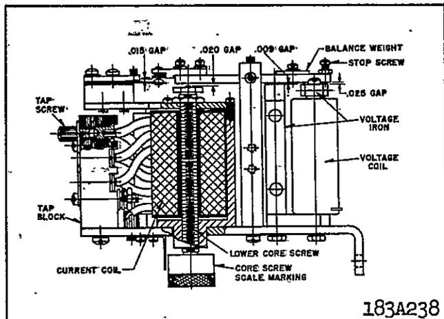
Fig. 1. Sectional View of the Impedance Units.
