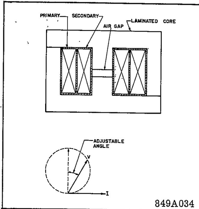
Fig. 4. Compensator Construction
