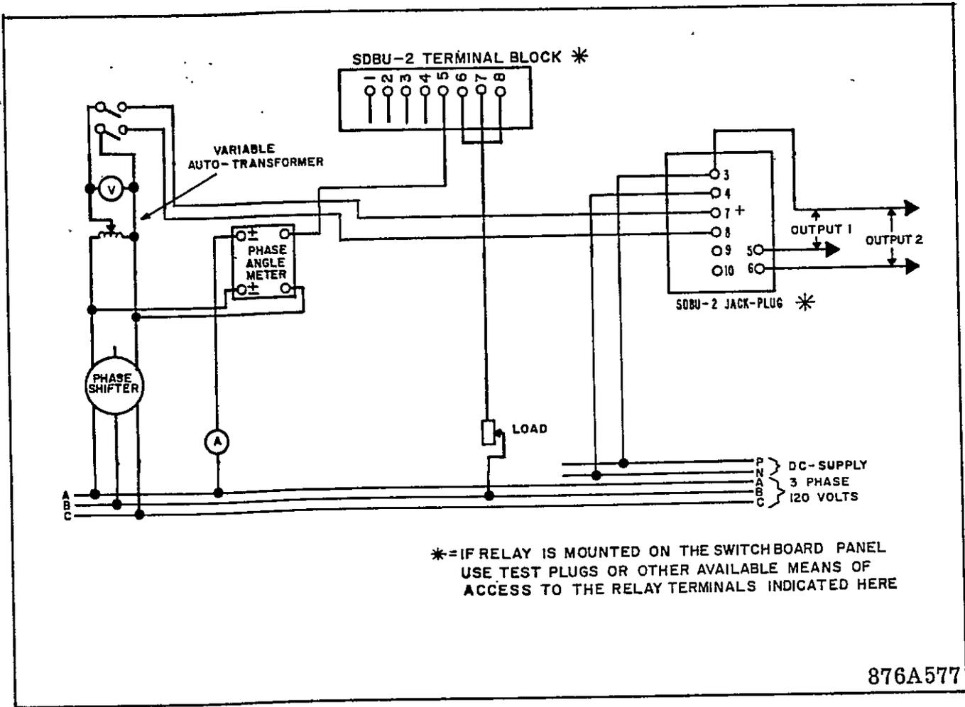
Fig. 15. Test Connections for SDBU-2 Relay
