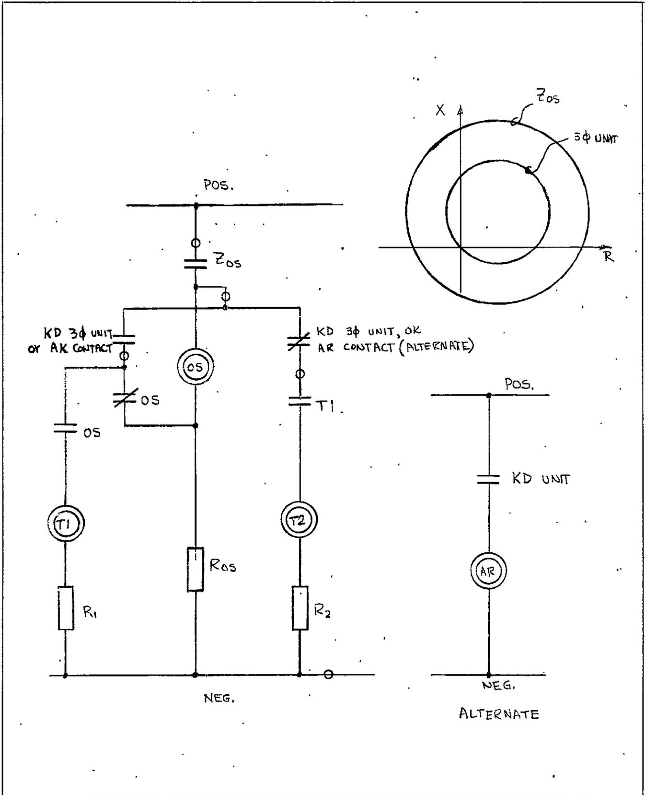
Fig. 4 Out-of-step Sensing Sequence
