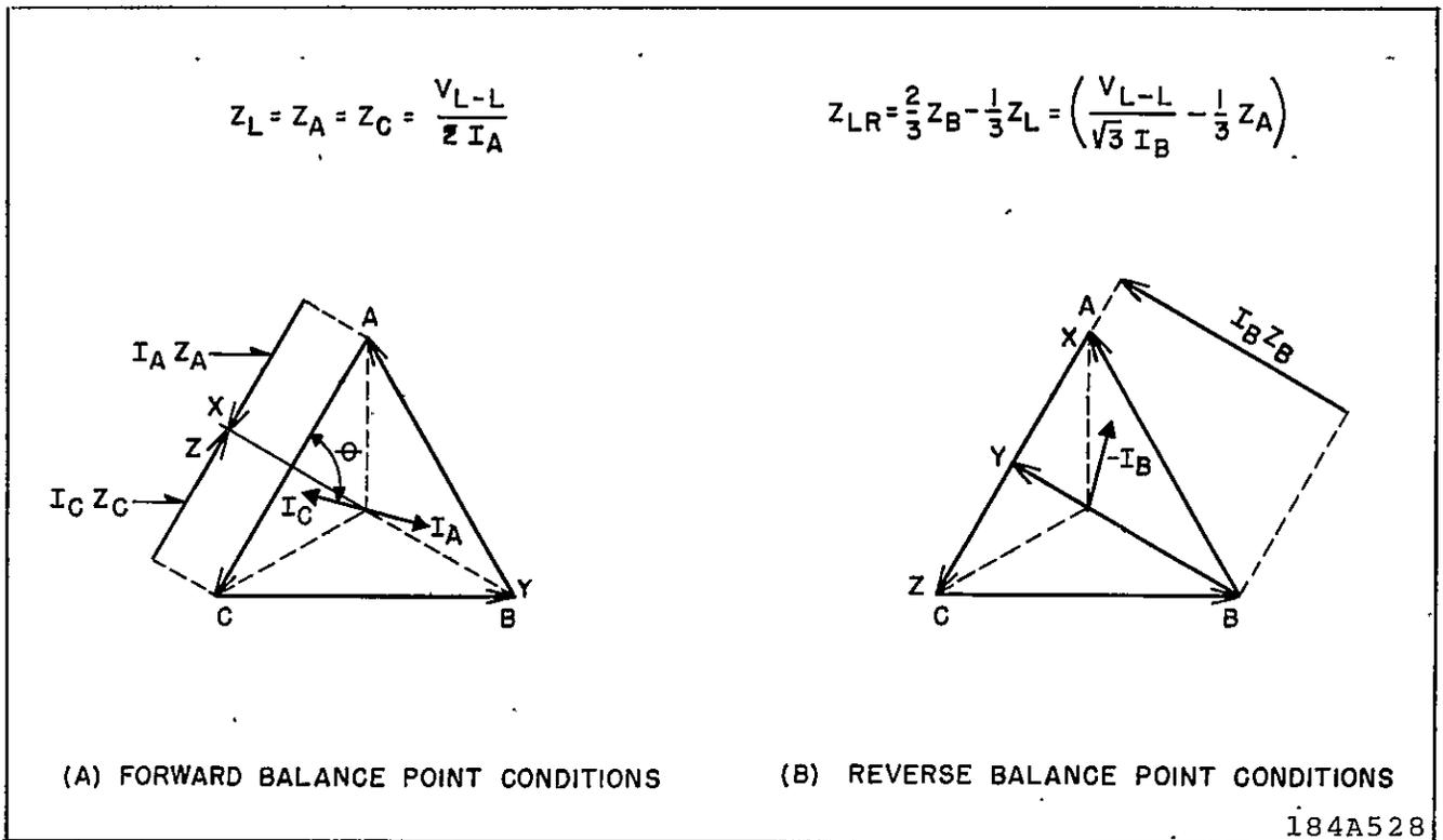
Fig. 8 Vector Diagram for the Artificial Reverse Balance Point Condition when Testing with Single Phase Current.
