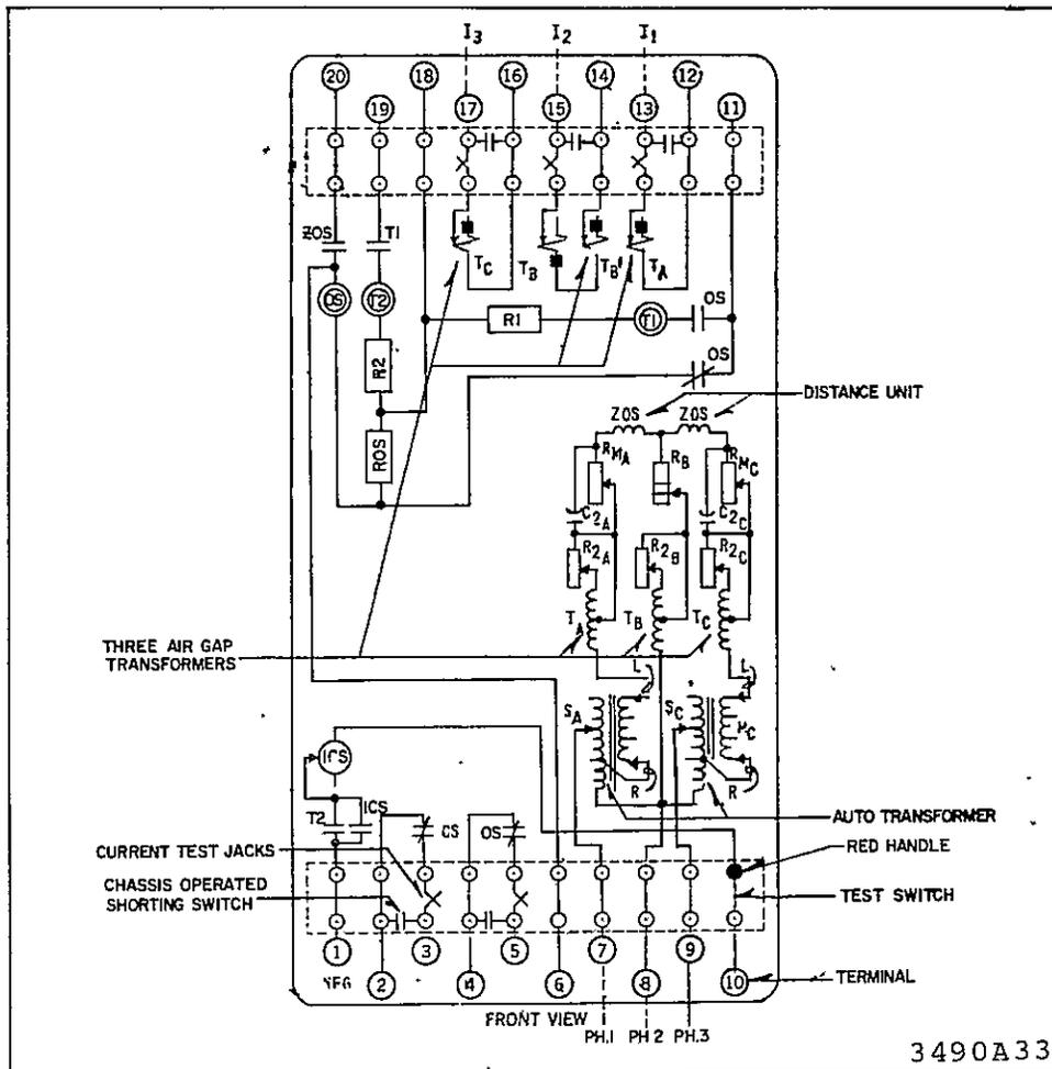
Fig. 3 Internal Schematic
