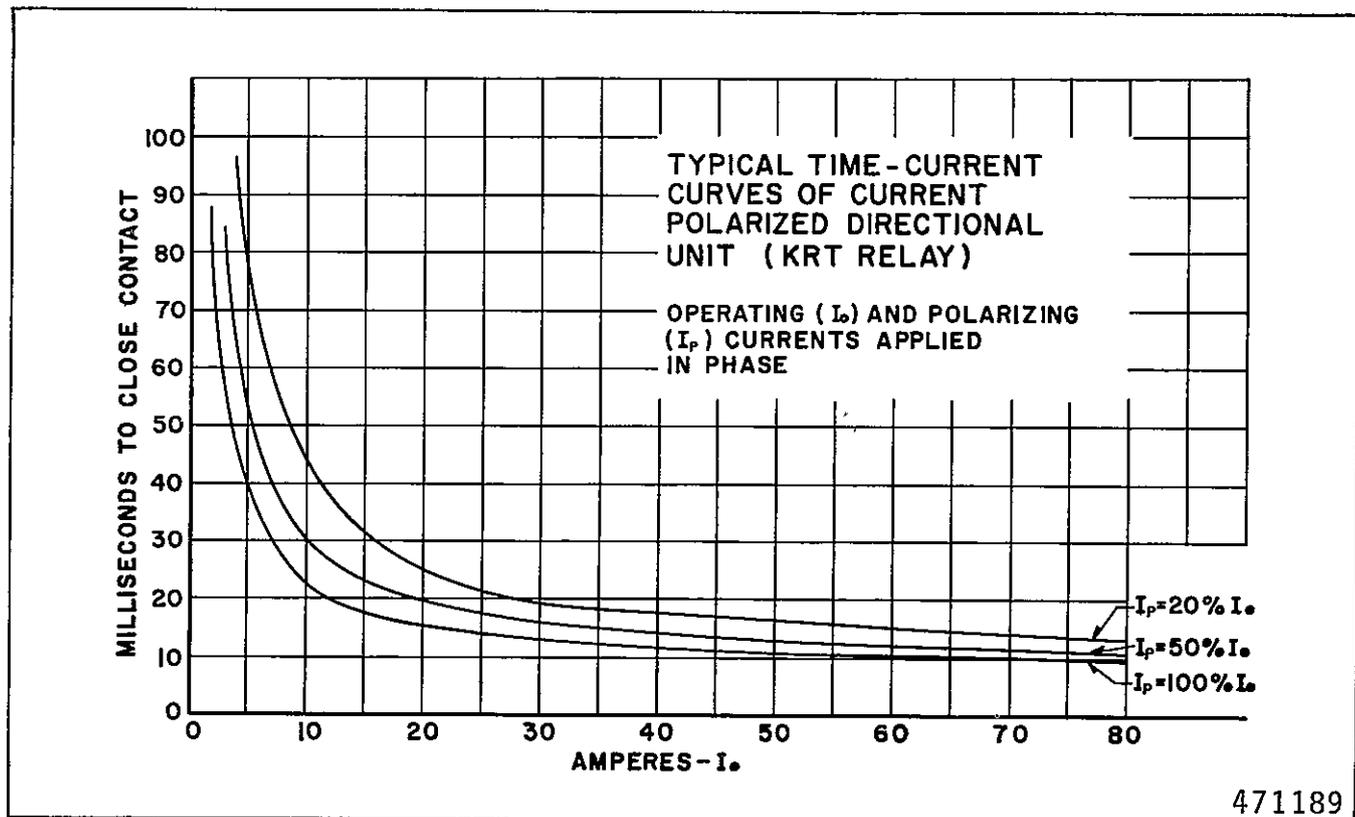
Fig. 4. Time Curve for Current Polarized Operation
