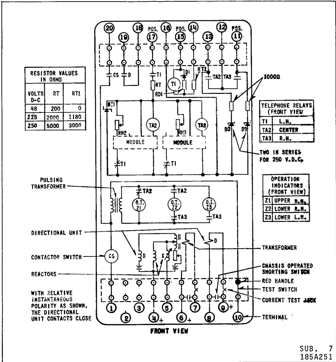
Fig. 1. Internal Schematic
