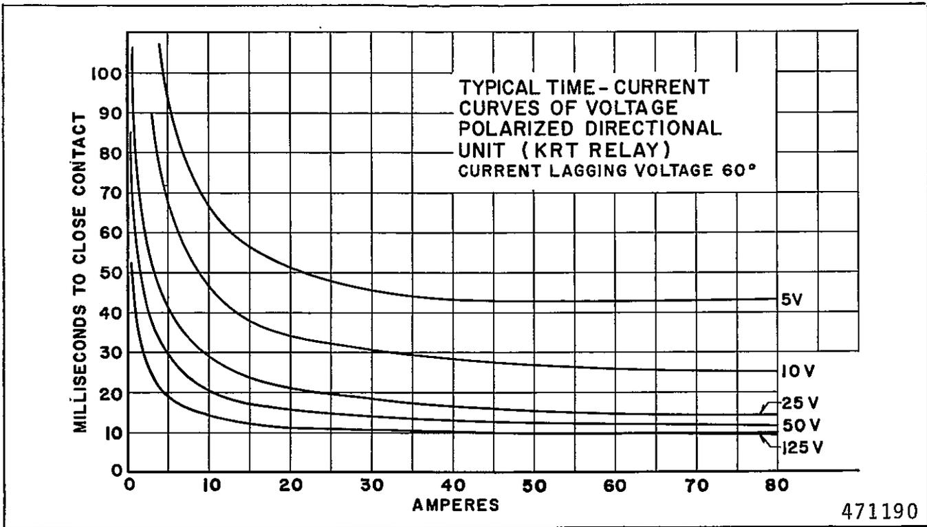
Fig. 5. Time Curve for Voltage Polarized Operation
