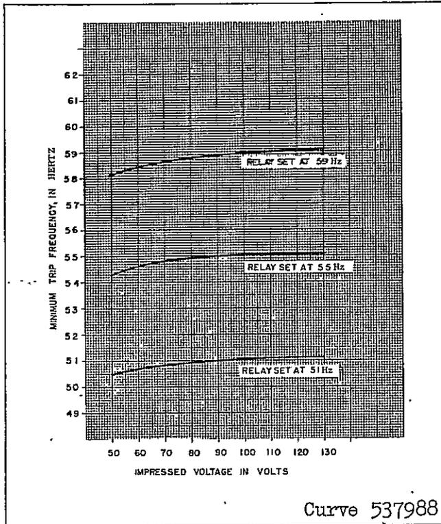
Fig. 3. Typical Voltage-Minimum Trip Frequency Curves of the Type CF-1 Underfrequency Relay.
