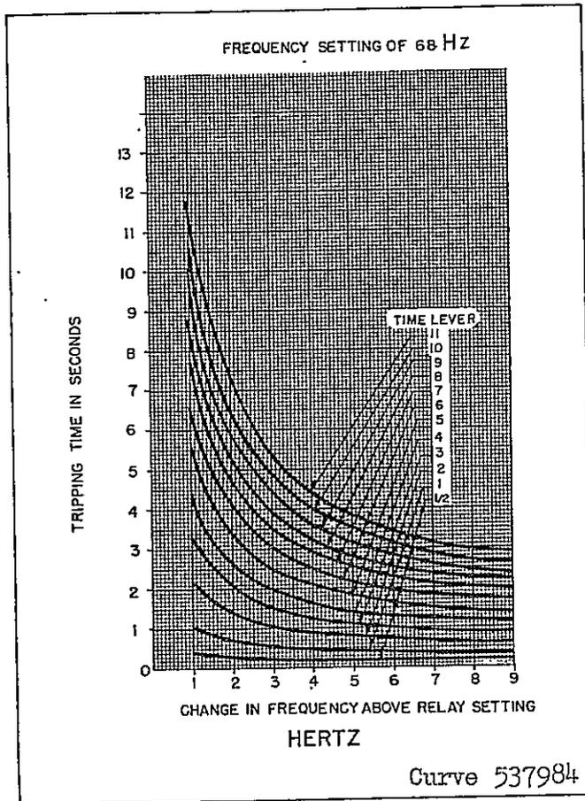
Fig. 10. Typical 68 Hz Time Curves of the Type CF-1 Overfrequency Relay.
