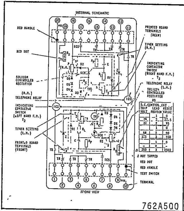
Fig. 2. Internal Schematic of Type TD-52 Relay with Single Trip 0.2/2.0 Ampere ICS Units (Relay with Single Trip 1.0 Ampere ICS Units has Identical Wiring Except the ICS Coils are not Tapped on Terminals 10 and 20, 849A417).
