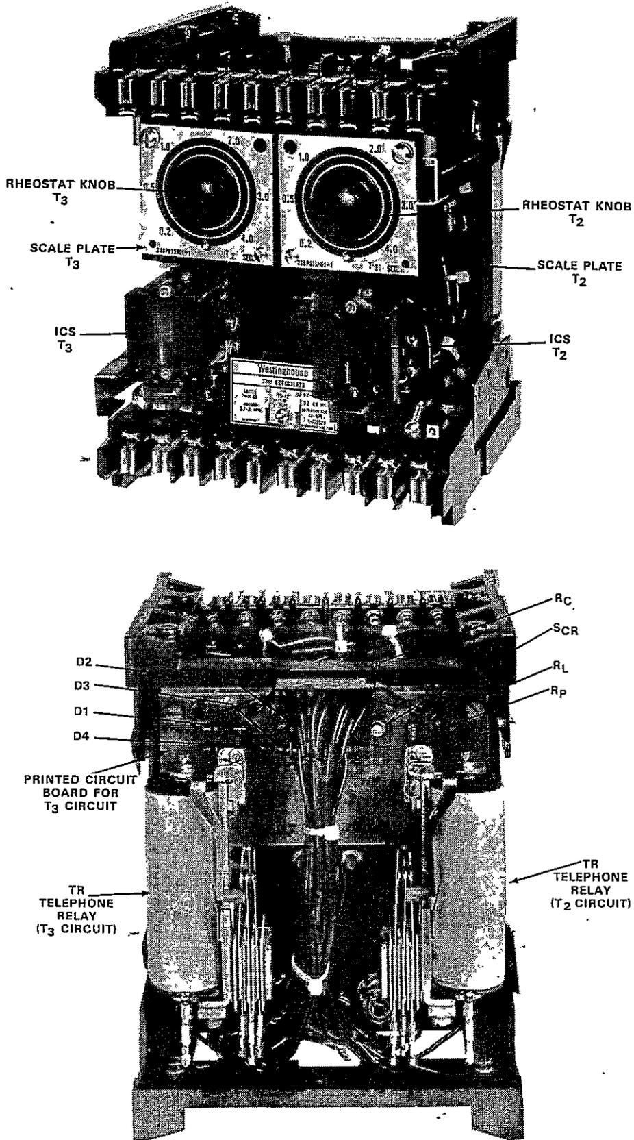
Fig. 1. Type TD-52 Relay Without Case.
