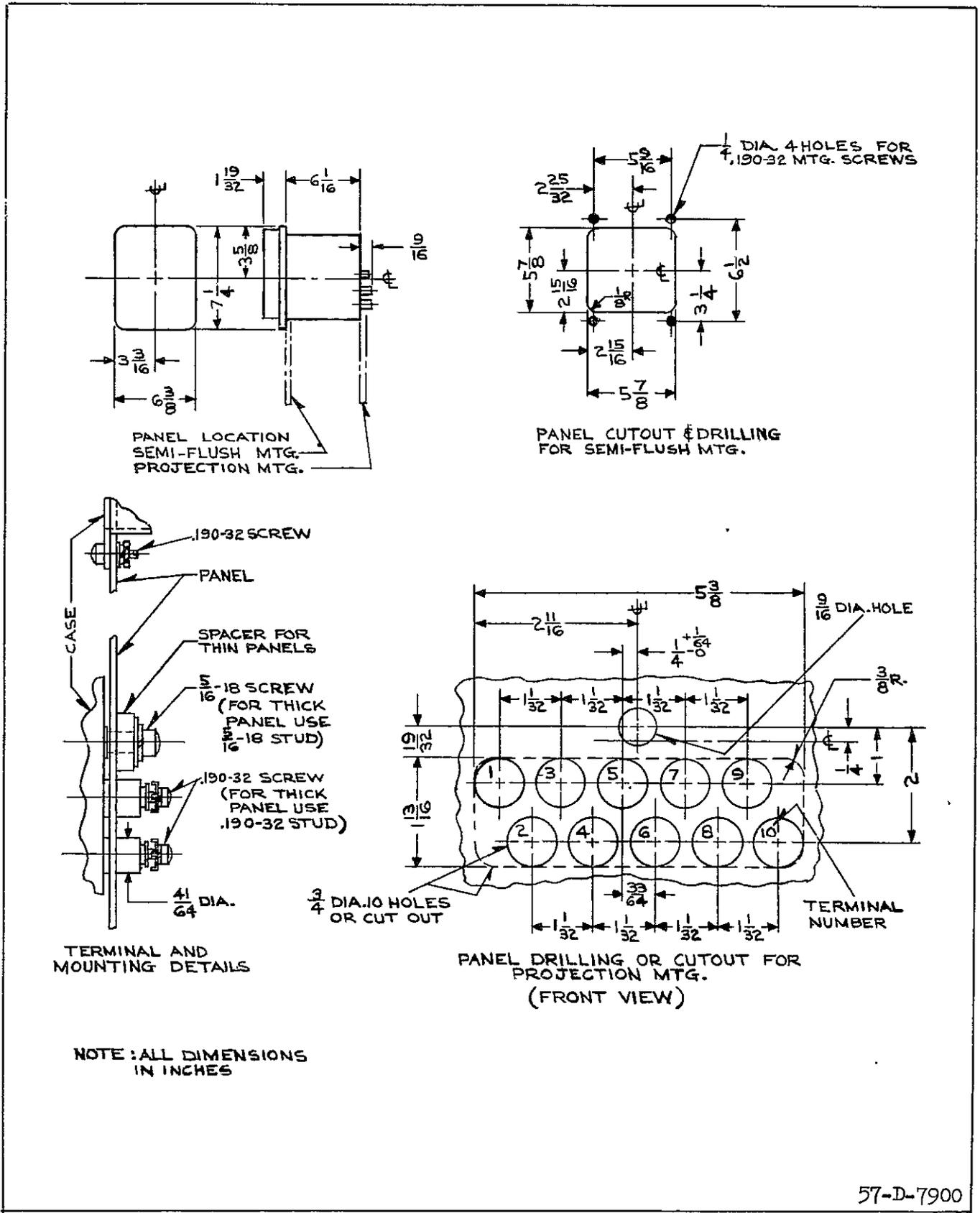
Fig. 6. Outline and Drilling Plan for the SGR-1 Relay in the FT11 Case.
