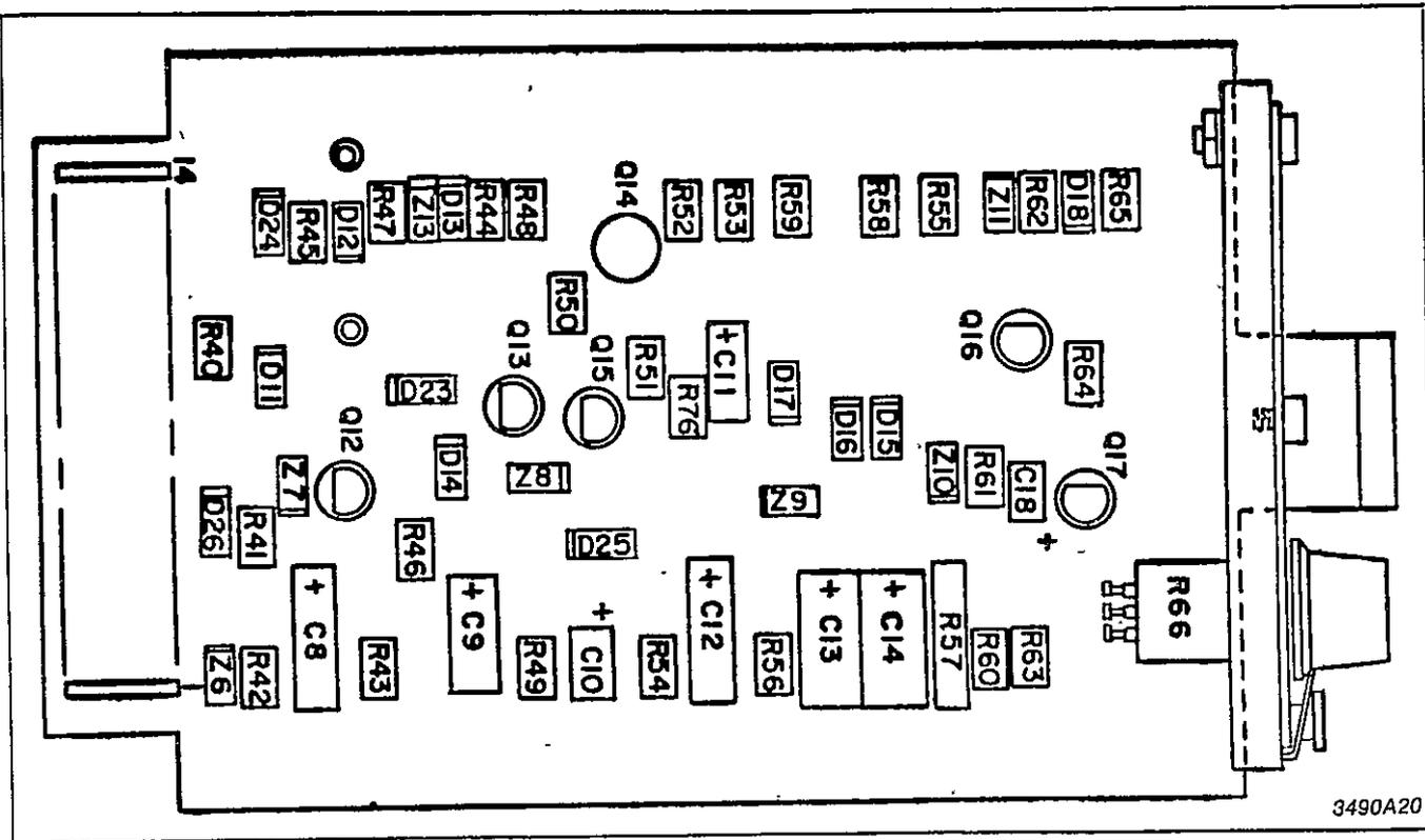
Fig. 6. Component Location of Reclose Printed Circuit Board for Type SGRU-52 Relay.
