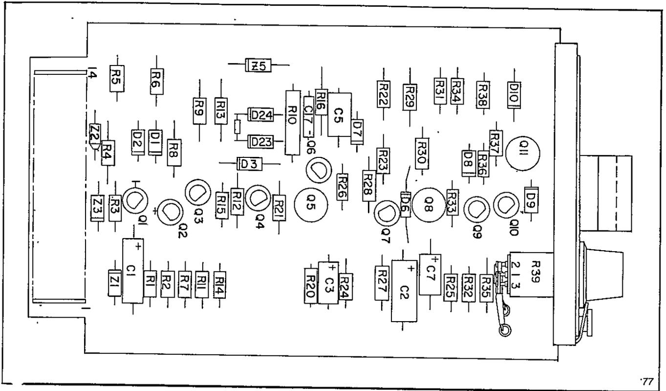
Fig. 7. Component Location of Reset Printed Circuit Board for Type SGRU-52 Relay.
