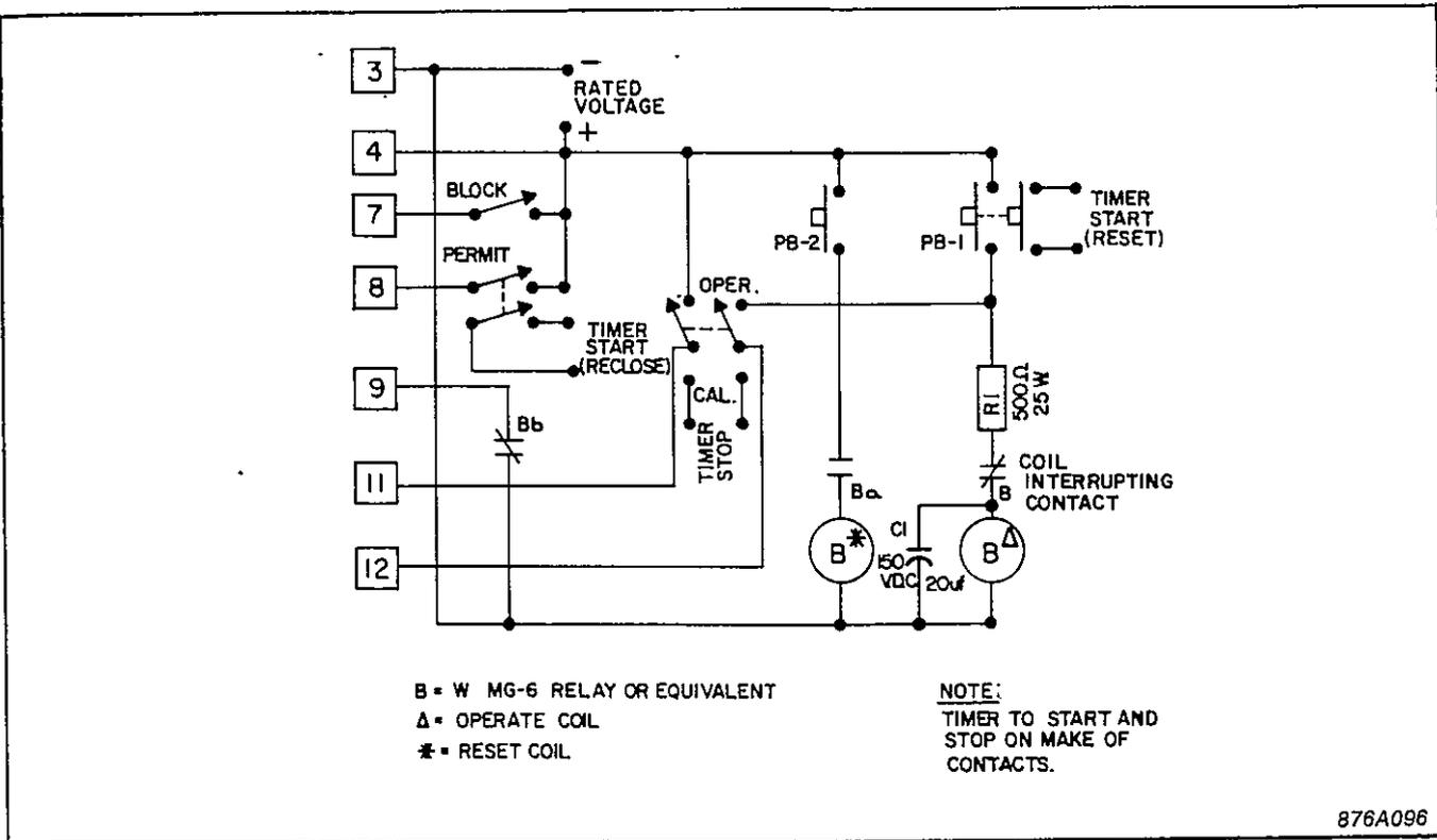
Fig. 5. Test Circuit of Type SGRU-52 Relay.
