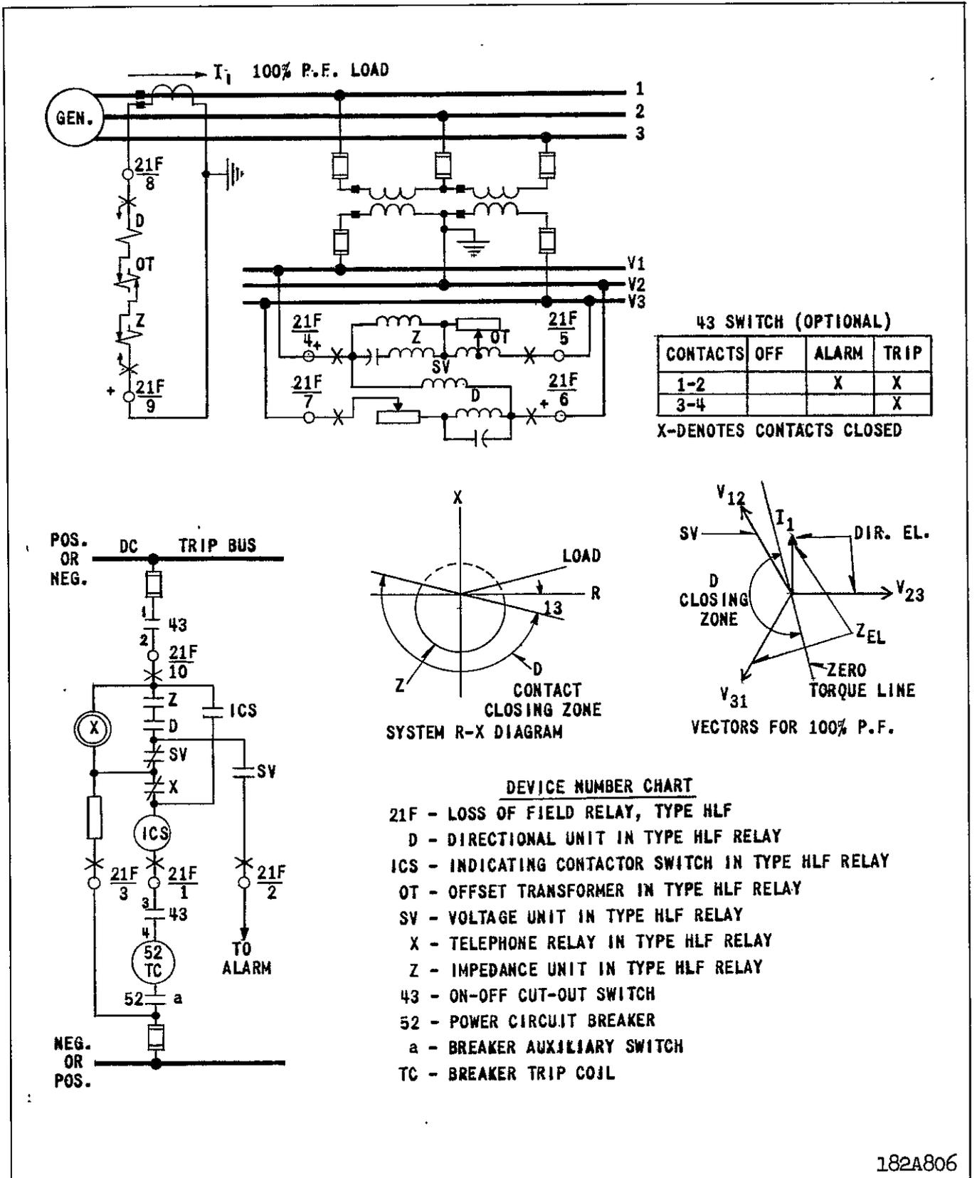
Fig. 3. External Schematic of the Type HLF Relay.
