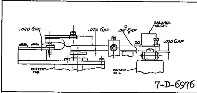
Fig. 1. Sectional View of Impedance Unit Beam.
