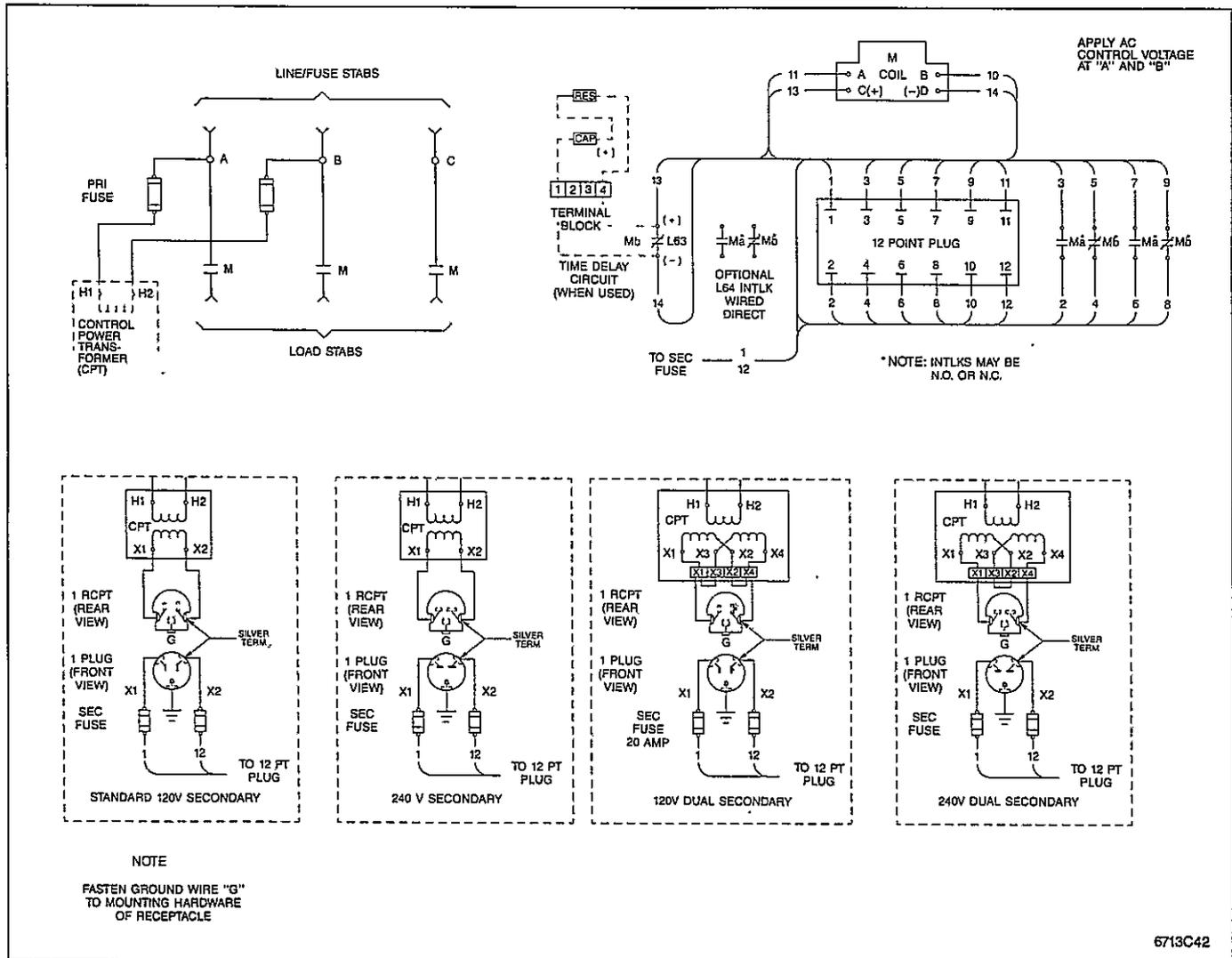
Fig. 8 Cable and Connection Diagram
