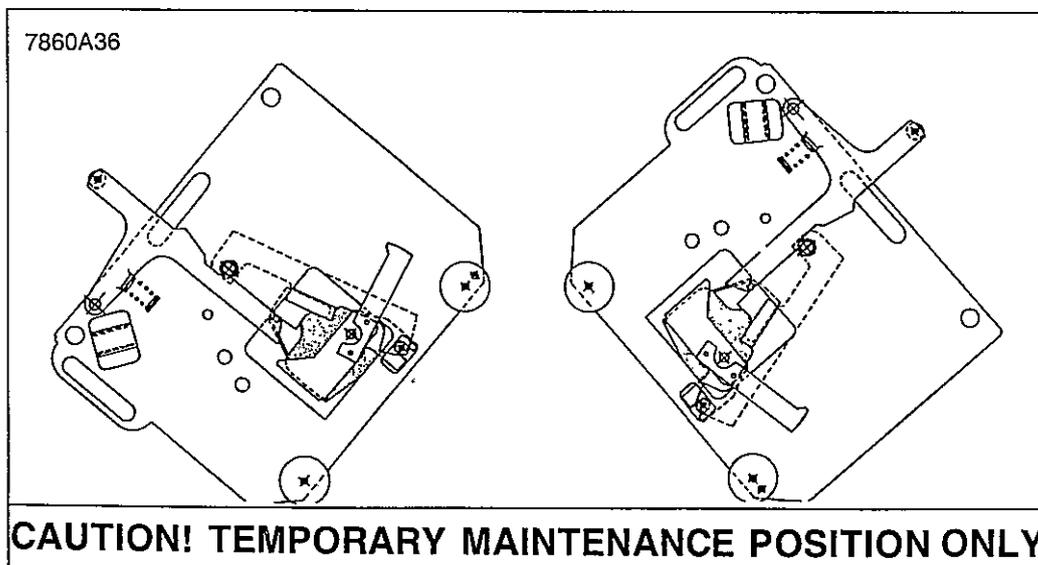
Fig. 5 Contactor Tilt Position
