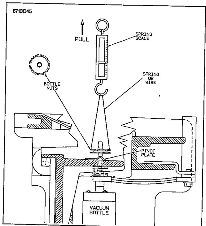
Fig. 6 Measuring Contact Force
