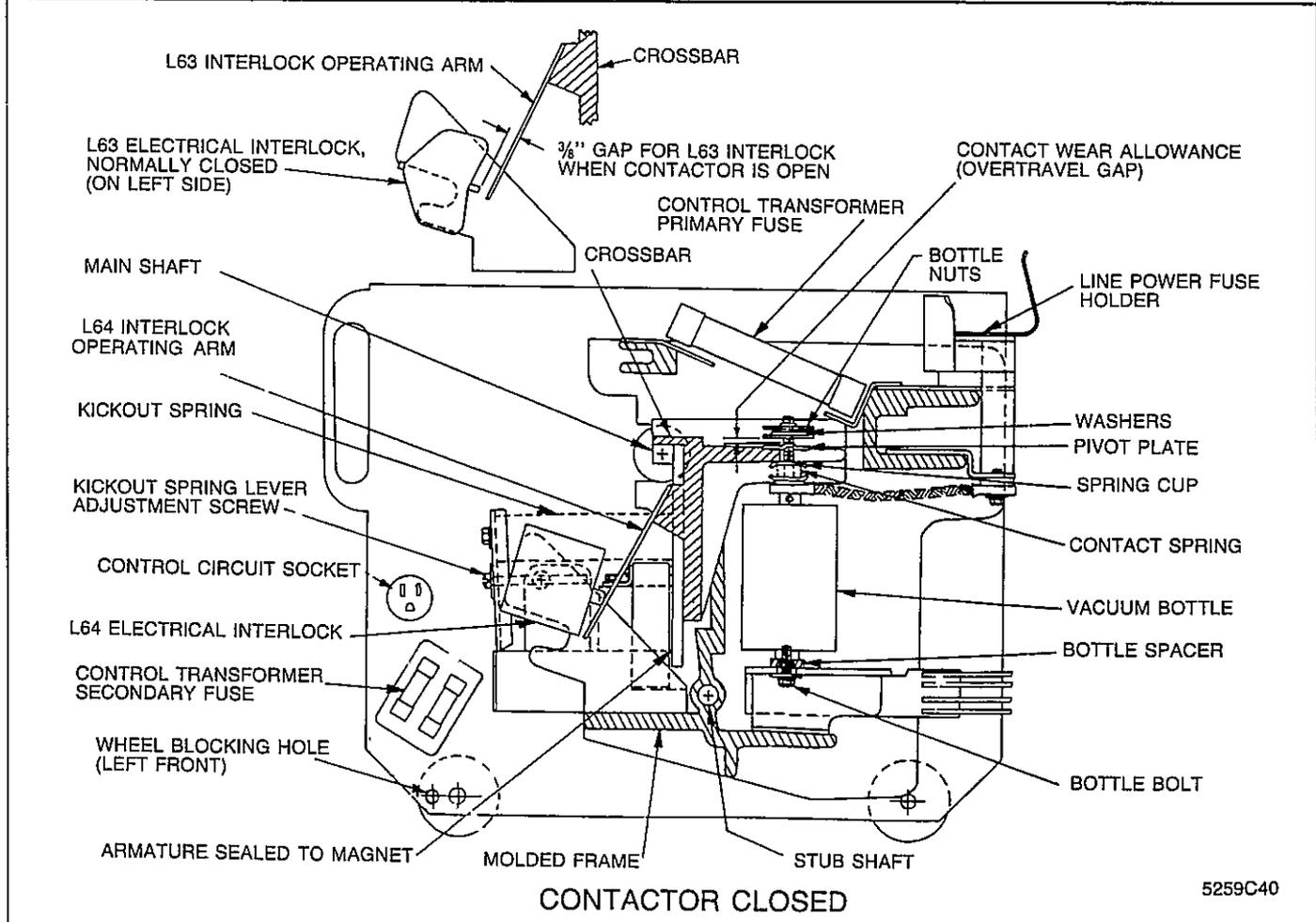
3 Fig. 4 Contactor Positions
