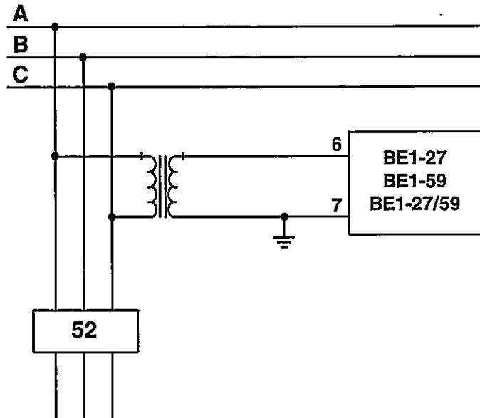
Figure 3. Voltage Sensing
