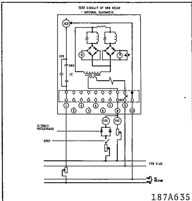
Fig. 8 Test Circuit (Single Phase HRU Relay).
