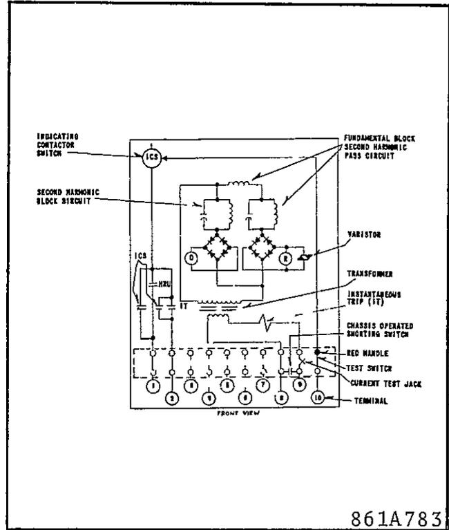
Fig. 2 Internal Schematic of Single Phase HRU Relay
