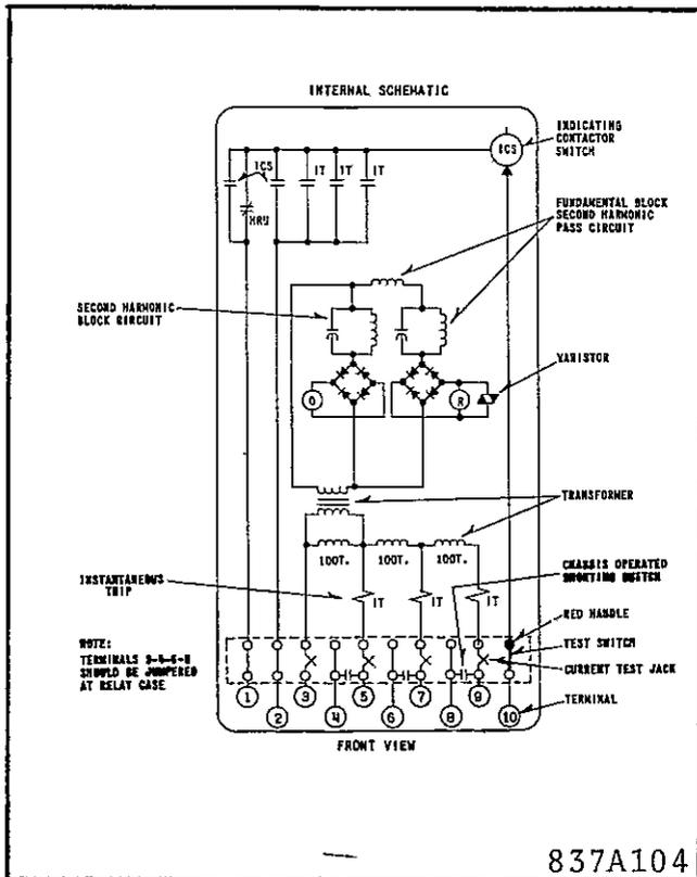
Fig. 3 Internal Schematic of 3-Phase HRU Relay
