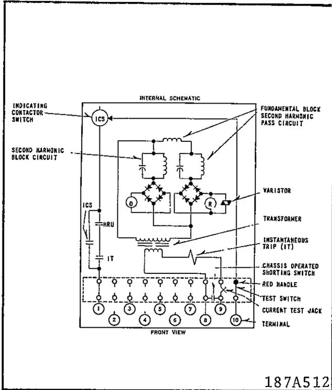
Fig. 1 Internal Schematic of Single Phase HRU Relay
