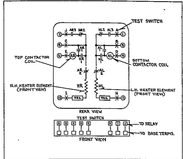
Fig. 8—Schematic Diagram of Type TH Duplex Relay.
