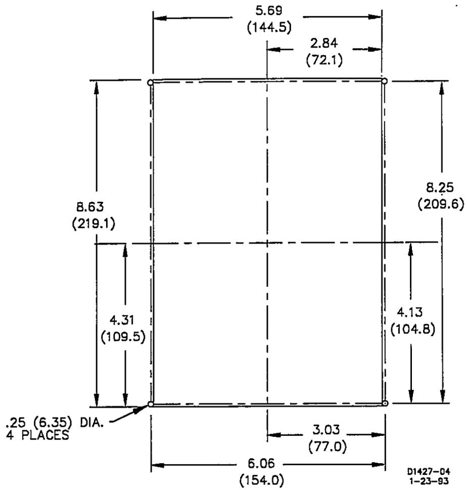
Figure 4-2. S1 Case, Panel Drilling Diagram, Semi-Flush Mounting
