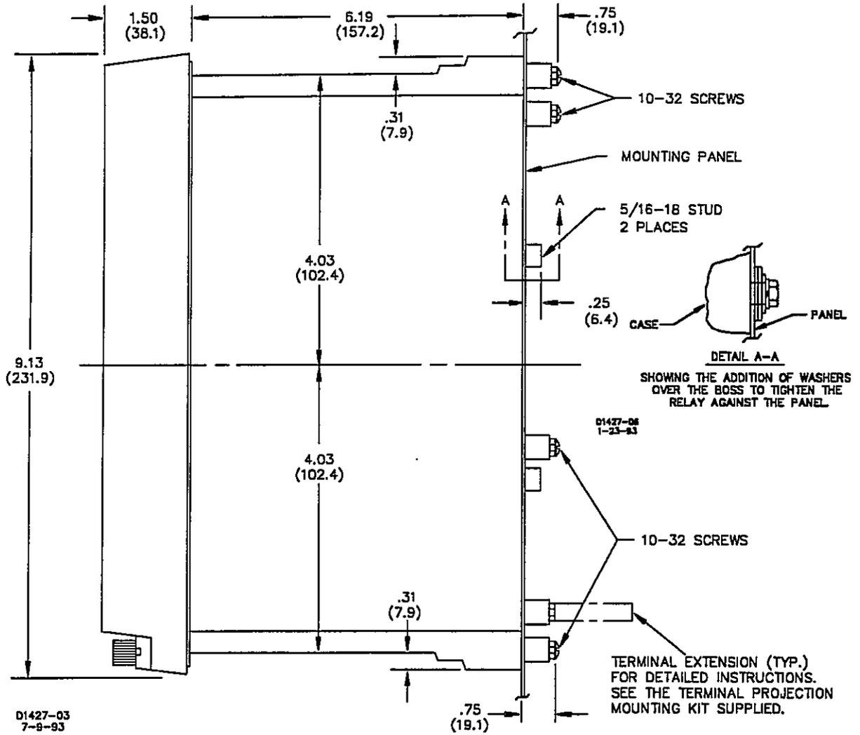
Figure 4-6. S1 Case, Double-Ended, Projection Mounting, Side View
