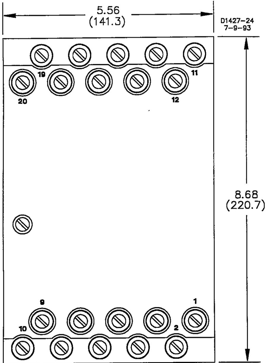
Figure 4-3. S1 Case, Double-Ended, Semi-Flush Mounting, Outline Dimensions, Rear View
