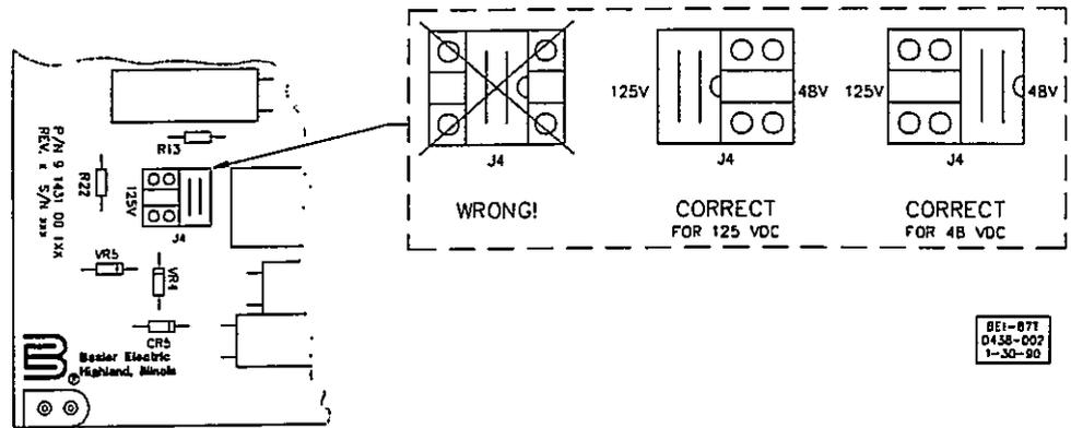
Figure 3-2. Power Supply Type S Link Position
