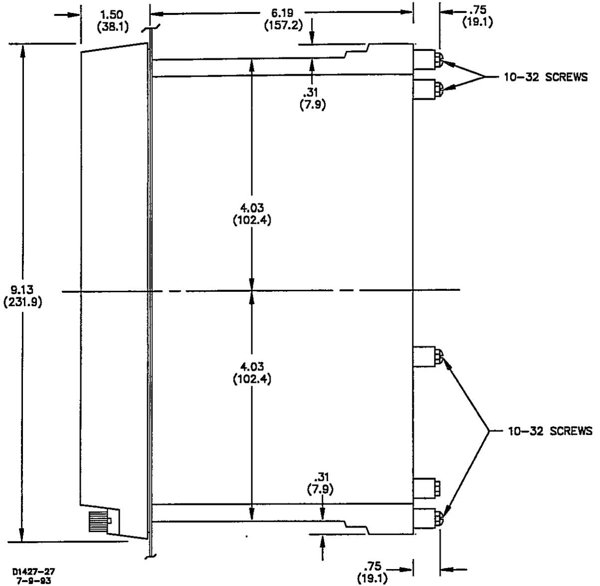
Figure 4-4. S1 Case, Double-Ended, Semi-Flush Mounting, Side View
