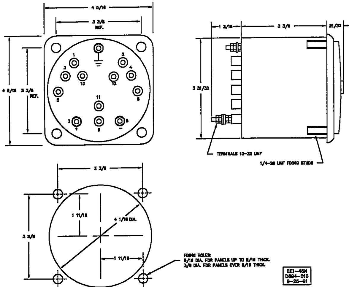
Figure 4-7. Remote Meter Dimensions and Drilling Diagram
