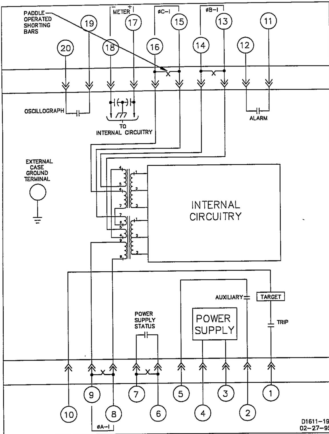
Figure 4-10. Typical Internal Connections
