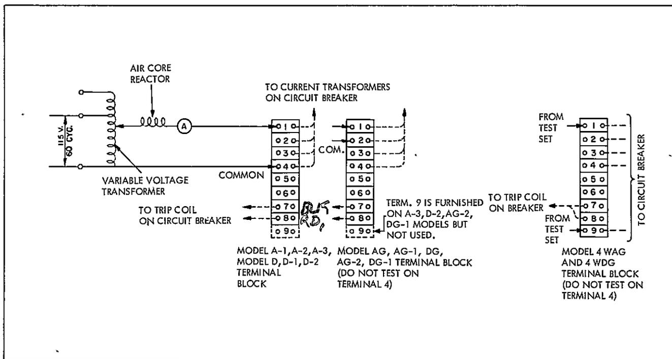
Fig. 8 — Connections for function tests.
